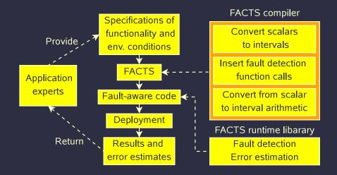
System overview Fault detection Error estimation Error propagation
